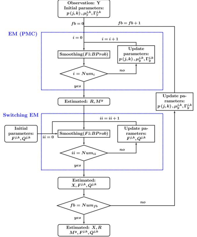
Fig. 1. Flowchart of DEM-CGPMSM.
