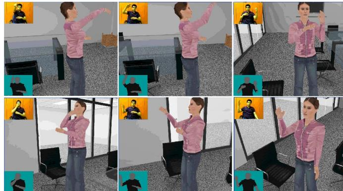
**Fig. 3.** Real-time 3D motion capture by computer vision and virtual rendering. For each captured image (top left inlays), the 3D model is projected with the pose that best matches the primitives (bottom left inlays). The virtual avatar (OpenSpace3D [11]) renders the captured gestures.
