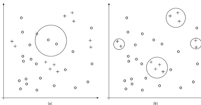
**Fig. 3.** A comparison between the TC behavior of (a) the Rocchio classifier, and (b) the  $k$ -NN classifier. Small crosses and circles denote positive and negative training instances, respectively. The big circles denote the “influence area” of the classifier. Note that, for ease of illustration, document similarities are here viewed in terms of Euclidean distance rather than, as is more common, in terms of dot product or cosine.
