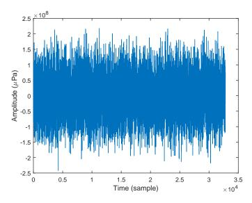
Fig. 4. Example output of simulated channel, with a distance of one km (signal amplitude ( $\mu$ Pa) as a function of time (sample).
