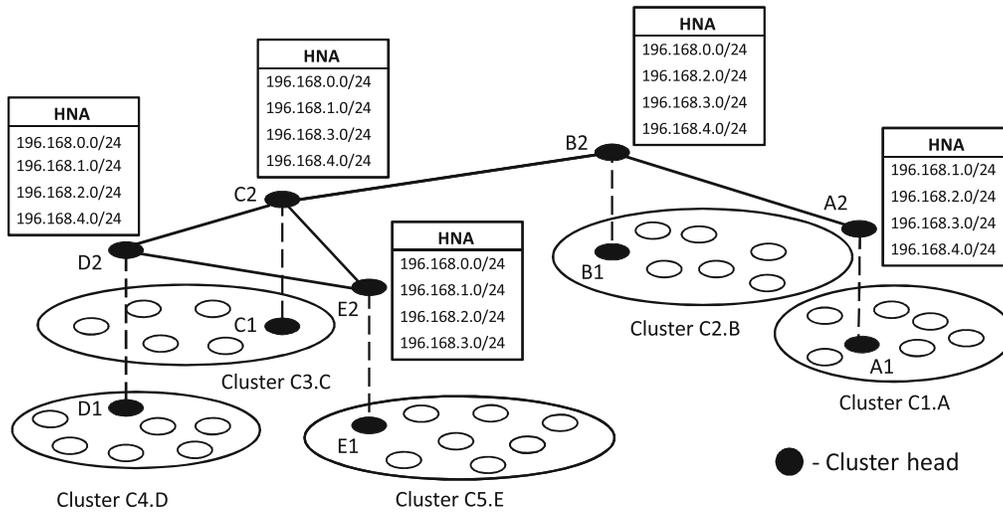
**Fig. 6.9** Example of a MORHE network. Consider *black nodes* as backbone nodes
