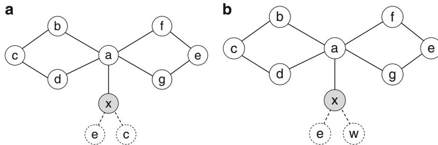
**Fig. 6.5** Flooding disruption due to link spoofing attacks. In Fig. 6.5a, node  $x$  spoofs links to nodes  $e$  and  $c$ . In Fig. 6.5b, node  $x$  spoofs links to nodes  $e$  and the inexistent node  $w$
