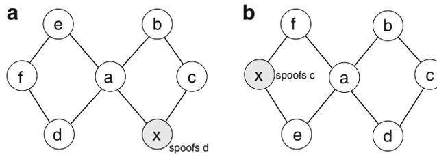
**Fig. 6.4** Flooding disruption due to identity spoofing attacks. In Fig. 6.4a node  $x$  spoofs  $d$  and reports an incorrect link between nodes  $c$  and  $d$  (one-hop address duplication). In Fig. 6.4b, node  $x$  spoofs  $c$  and affects node  $a$ 's MPR selection (two-hop address duplication)
