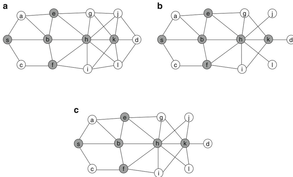
**Fig. 6.13** Network topology perspective of node  $s$ . Gray nodes represent MPRs. (a) Complete network topology. (b) Node  $s$  perspective of the network. TC\_redundancy equal to 0. (c) Node  $s$  perspective of the network. TC\_redundancy equal to 2
